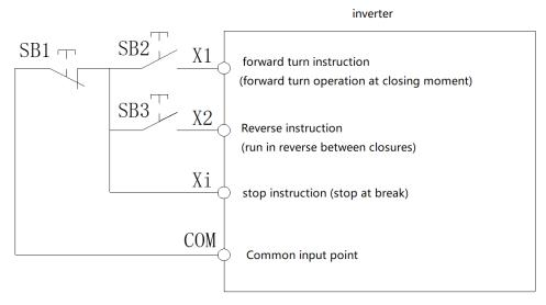
Three-wire system control 2 schematic diagram
