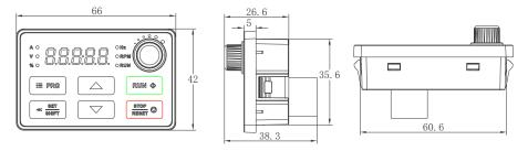
Boundary Dimension of Externally Single-line Keypad
