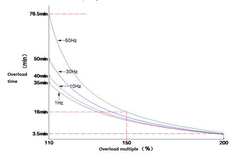
The overload protection curve under different frequency when the default is F level.
