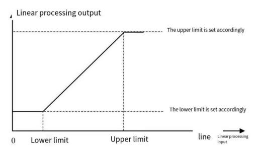
Schematic of Al Linear Processing
