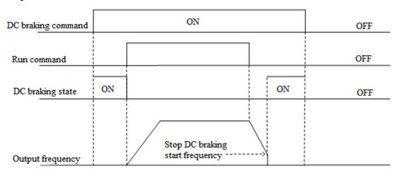
Schematic of DC Braking Command
