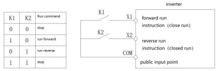
Schematic diagram of two-wire system control 1
