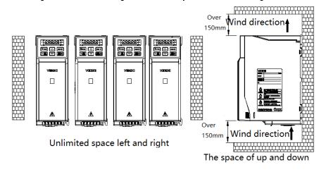
Figure 3-3: Inverter installation space requirements
