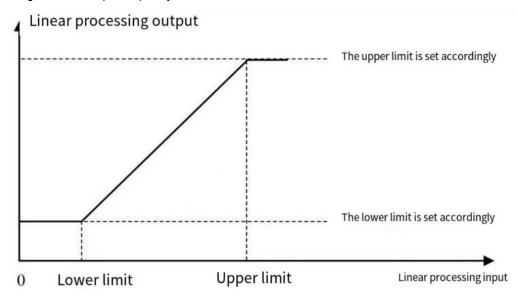
Schematic of Linear Processing of PUL Input Frequency
