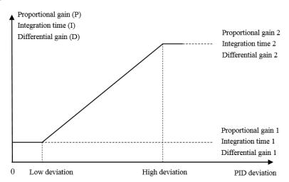
Diagram of deviation-based PID parameter changeover
