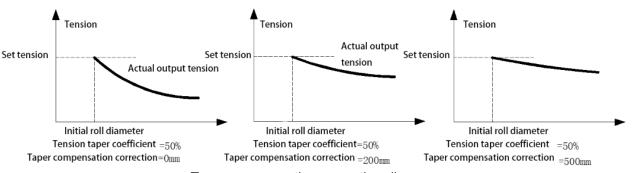
Taper compensation correction diagram
