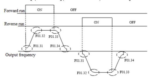
Diagram of S-Curve Characteristics
