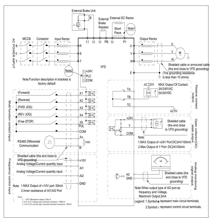
Figure 3-4: Standard connection diagram
