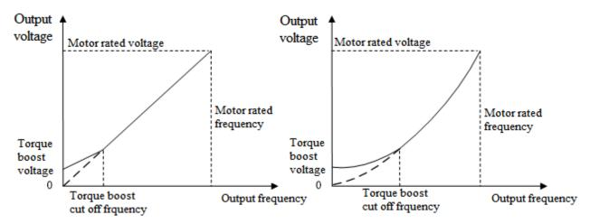
Schematic of Fixed Torque Boost
