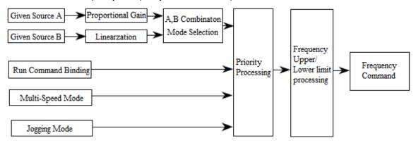
Diagram of Frequency Command Setting
