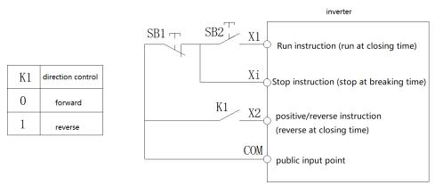
Schematic diagram of three-wire system control 1
