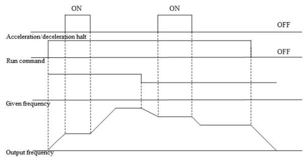
Schematic of Acceleration/Deceleration Halt
