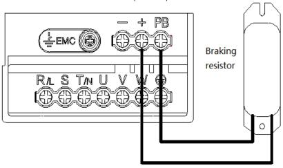
Figure 3-5: Connection diagram of braking resistor for AC310 series inverter below 22 kW (inclusive)
