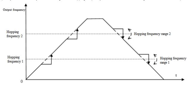
Schematic of Hopping Frequency Action
