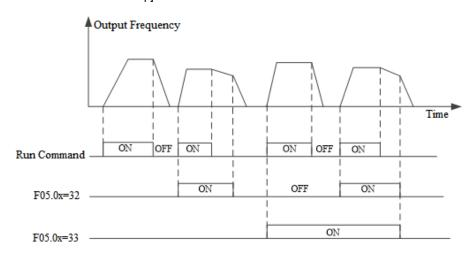
Time Sequence Diagram of Acceleration/Deceleration Time
