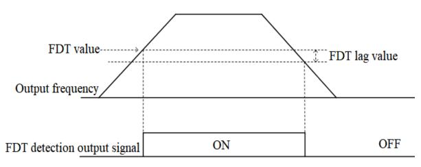
Schematic of Frequency Detection
