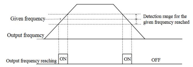
Schematic of Frequency Reaching Detection
