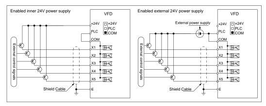
Wiring method of NPN characteristic transistor:
