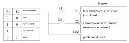
Schematic diagram of two-wire system control 2
