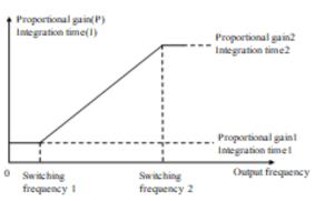
Diagram of Setting of Speed Loop Proportional Gain and Integral Time
