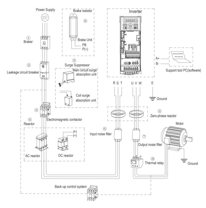
Figure 9-1: Connection block diagram of external devices
