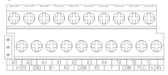
Table 3-6: Arrangement and definition of terminals of AC310 series inverter control circuit
